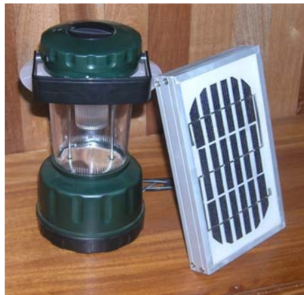
8pc solar LED lantern that has been imported for testing by a Ghanaian solar installer who is now investigating local assembly of the product
